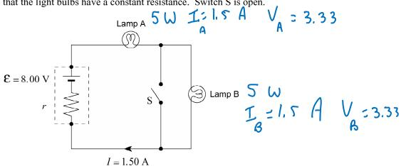
a) If a current of 1.50 A flows in the circuit, what is the internal resistance r of the battery?
