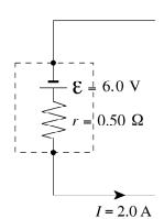
What will be the reading on a voltmeter connected to the battery terminals?
