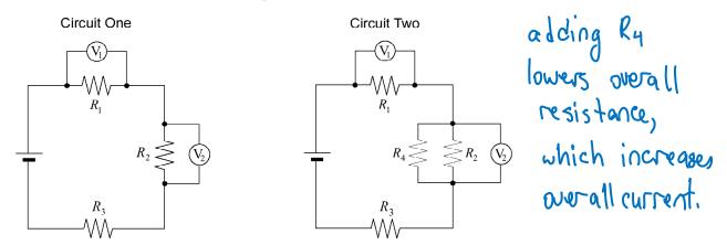
How have the values of  $V_1$  and  $V_2$  in circuit two changed compared to those in circuit one?
