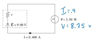
a) If a current of 0.400 A leaves the battery, what is the internal resistance, r, of the battery? (5 n
