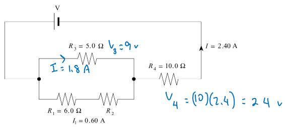
b) Find the potential difference of the power supply, V.
